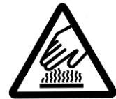
Caution: Burn Hazard!
